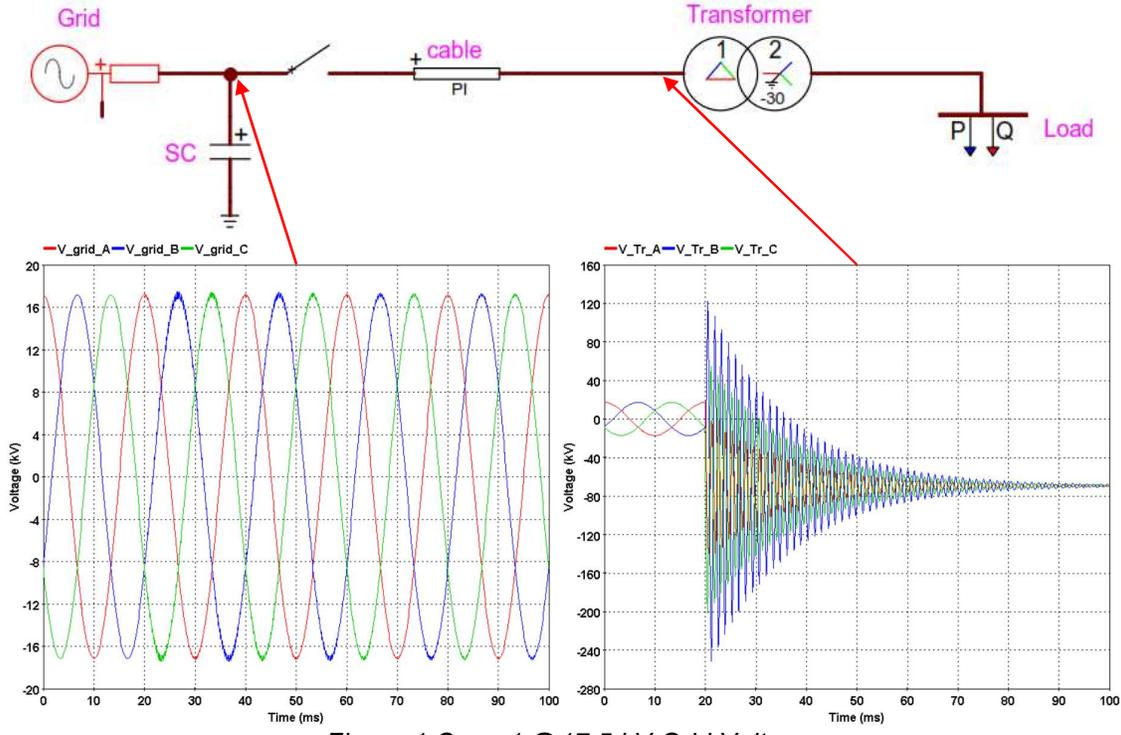
In CASE-2 where the surge capacitor is used for transient voltage waveform steepness and peak reduction on the transformer side, the defined withstand voltage limit in the standards are not exceeded and the oscillations in the transient voltage waveform are significantly reduced, but spikes occur on the grid voltage side.
