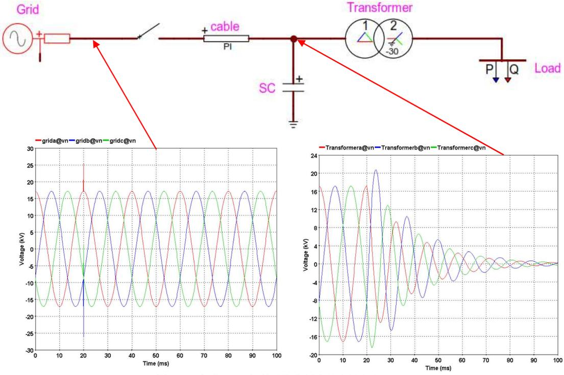
In CASE-3, where the surge capacitor is used for transient voltage waveform steepness and peak reduction at the both (Grid & Transformer) side, the defined withstand voltage limit in the standards are not exceeded and the oscillations in the transient voltage waveform are significantly reduced.
